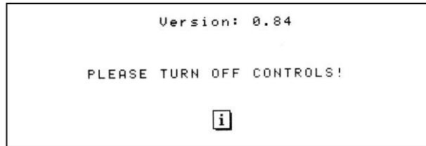
In order to eliminate the error, the intensity control has to be turned off.
