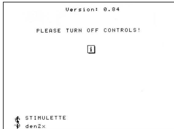
The intensity control has to be turned down until a click is heard (control is turned off). Then the device continues with the self-test.
